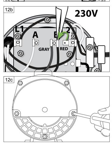
c. Reinstall the rear motor cover. (Fig.12c)
