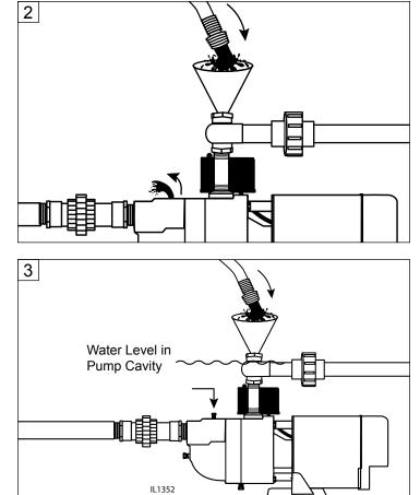
3. Replace air relief plug and continue adding water to pump cavity until water reaches the top of the priming plug. (Fig. 3)
