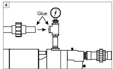
4. Continue with fittings and pipe to the pressure tank. A 3/4 in. union (optional) is recommended for easy connection and disconnection. (**Fig. 4**)
