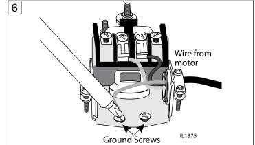
6. Connect the green ground wire from the motor cable to one of the green ground screws at the bottom of the pressure switch. (Fig. 6)
