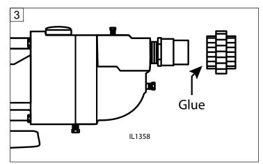
3. The use of a union (optional) will assist with easy connection and disconnect. (**Fig. 3**)
