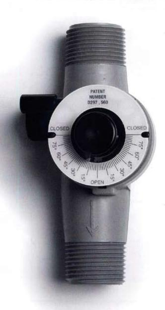
The WellMate Micronizer installs easily to any hydropneumatic tank, drawing air into the water line through the air inlet. When properly installed and adjusted, the Micronizer will continually charge the tank with air for 30% to 50% of the pump's run time. Excess air is relieved through an AVC assembly installed in the tank.
