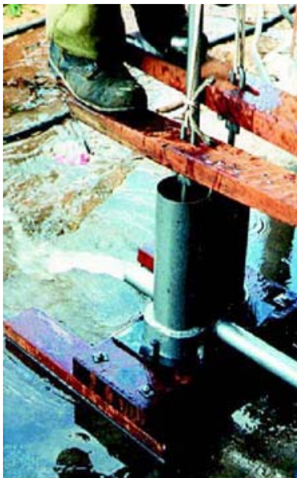
Figure 8: Masvingo treadle pump (pressure delivery), under test at manufacturers
