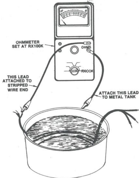
Ohmmeter connections for cable and splice test.
