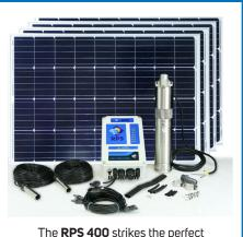
balance between cost and performance. It comes standard with four 100 watt solar panels, a 'smart' controller, wires and sensors. It can operate at a maximum head of 262 feet and generates flow rates up to 7.9 gallons per minute. The RPS 400V+ with centrifugal pump
