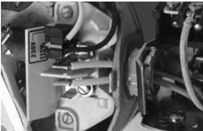
Figure 9: Voltage set to 115 volts, Plug Type
