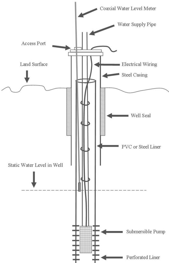
**Above:** Measuring water levels in wells with liners can be difficult. To get an accurate reading you must be sure that you are inside the liner. You also must be careful to avoid wiring or other potential hang-ups.
