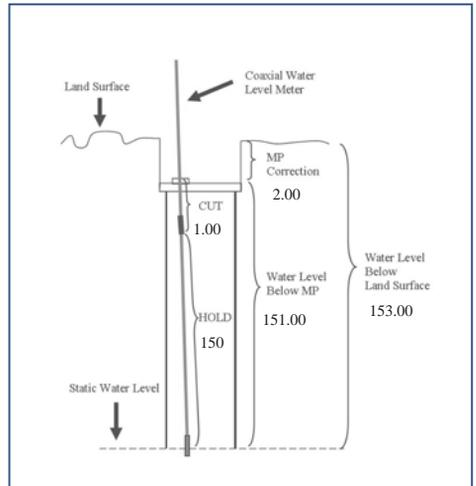
\*To prevent surface water from contaminating your well, all well casing should rise at least 12-inches above land surface according to Oregon Well Standards.
