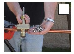
**Step 2**Disassemble the Add-A-Valve® body by removing the four (4) 316 stainless steel bolts.
