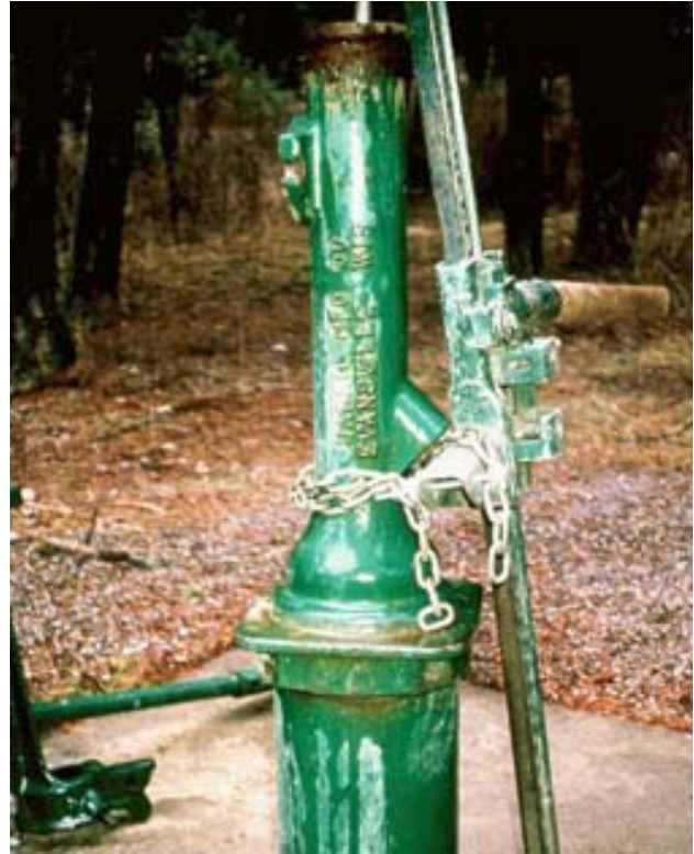
Figure 17—View of the chain securing the jack to the pump base.
