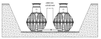
tanks is at least 600 mm (23.62 inch). The pipes must project at least 200 mm (7.87 inch) into the tanks.
