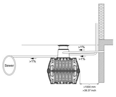
Important: The empty pipe must be connected to an opening above the max. water level.
