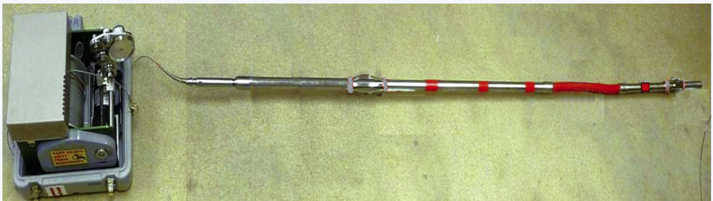
Figure 5. Full-waveform sonic (FWS) tool attached to cable with winch. The transmitter is the short red section at the bottom of the tool to the right. The receivers are the three short red sections in the middle of the tool. The longer red section separating the transmitter from the receiver array is an acoustic isolater made of rubber.
