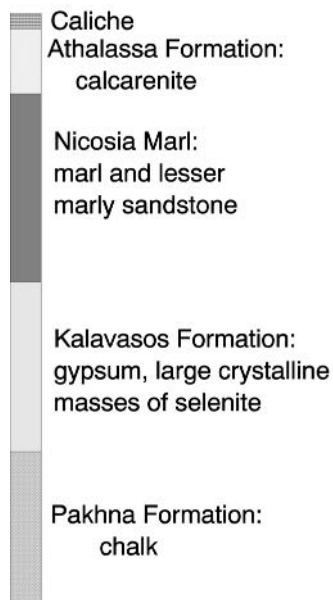
Figure 2. Generalized stratigraphic column for the Pergamos, Cyprus area, based on logs of drilled wells and a hand dug well that penetrated gypsum. Not to scale; see text for approximate thicknesses.
