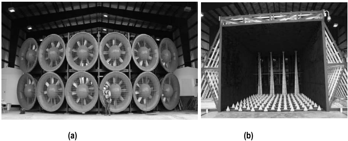
Figure 1: Wall of Wind (a) upstream view and (b) downstream view
