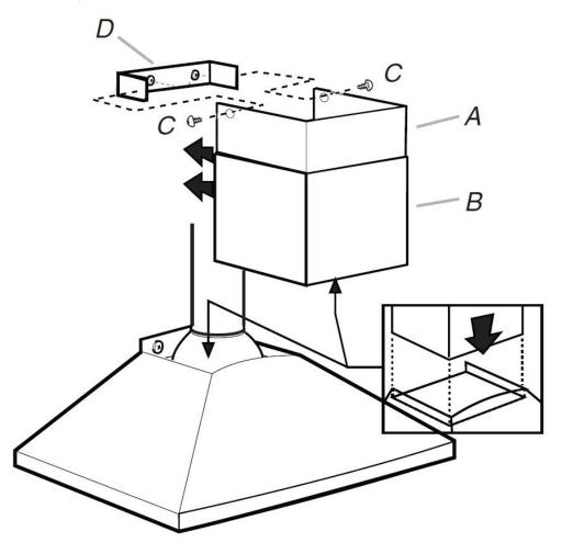
**NOTE:** For vented installations, the upper vent cover maybe reversed to hide slots.
