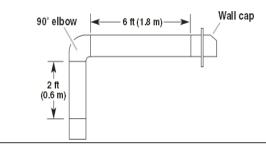
The following example falls within the maximum recommended vent length of 35 ft (10.7 m).
