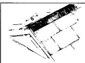
4. Mark end of slot 6" from inside of end wall. See illustrations for special applications.
