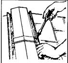
9. Place straps over joints and fasten in place. Use connector straps at each end of vent run.
