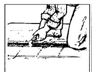
5. Cut through shingles to roof sheathing with utility knife.
