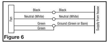
Carefully tuck wires back inside wire compartment and replace wire compartment cover securing with the screw that was removed earlier.
