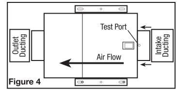
Ensure duct joints and exterior penetrations are sealed with caulk or other similar material 2. to create an air-tight path to minimize building heat loss or gain and to reduce the potential for condensation. Place/wrap insulation around duct and/or fan in order to minimize possible condensation buildup within the duct, as well as building heat loss or gain.
