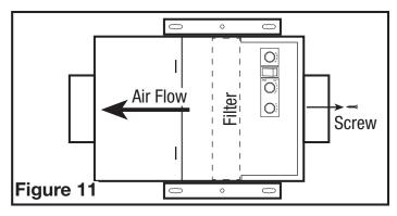
3. Close the access panel and reinstall the screw holding the access panel in place.
