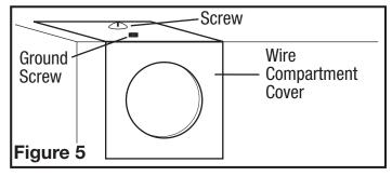
2. Pull the loose black, white and green wires out from the wire compartment (additional wires will be present). Install an approved electrical connector to the wire compartment cover (not included). Run a black (hot), white (neutral), and a green or bare ground wire from the supply through the electrical connector. Connect all wires from the supply to their corresponding wires within the wire compartment (Figure 6). Use approved methods for all connections.
