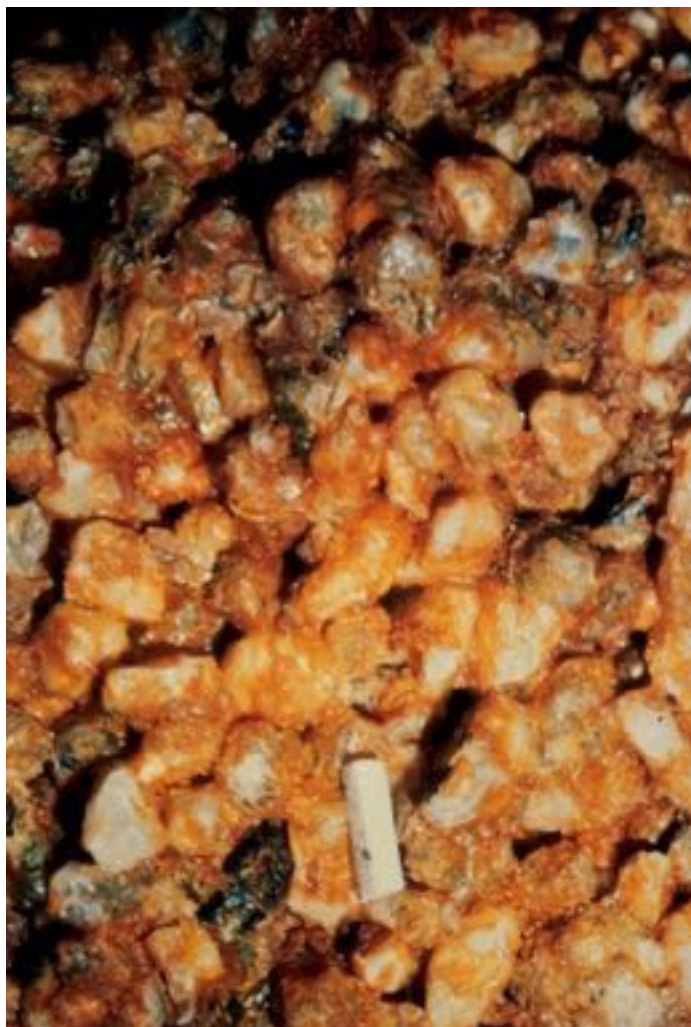
Photo 15.—Clay films and bridges on sand grains, which commonly occur in argillic horizons with associated eluvial horizons that have less than 15 percent clay.
