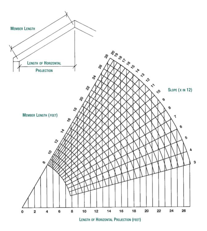
Spans given in the tables are the maximum allowable horizontal span of the member from inside to inside of bearings. For sloping rafters, spans are measured along the horizontal projection. This diagram provides a convenient tool for calculating the corresponding sloping distance of a rafter. Select the horizontal span along the horizontal axis and follow the vertical line upward to its intersection with the radial line of the specified slope. Then follow the arc line
