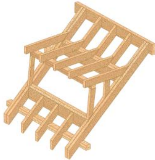
Figure 10-128 – Framing a shed dormer.
