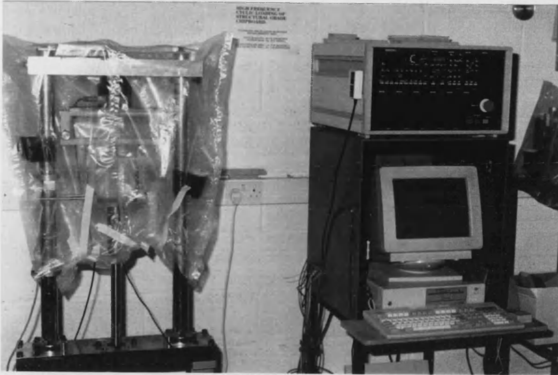
Fig 6.3 Dartec fatigue rig, controller and fatigue data acquisition system.
