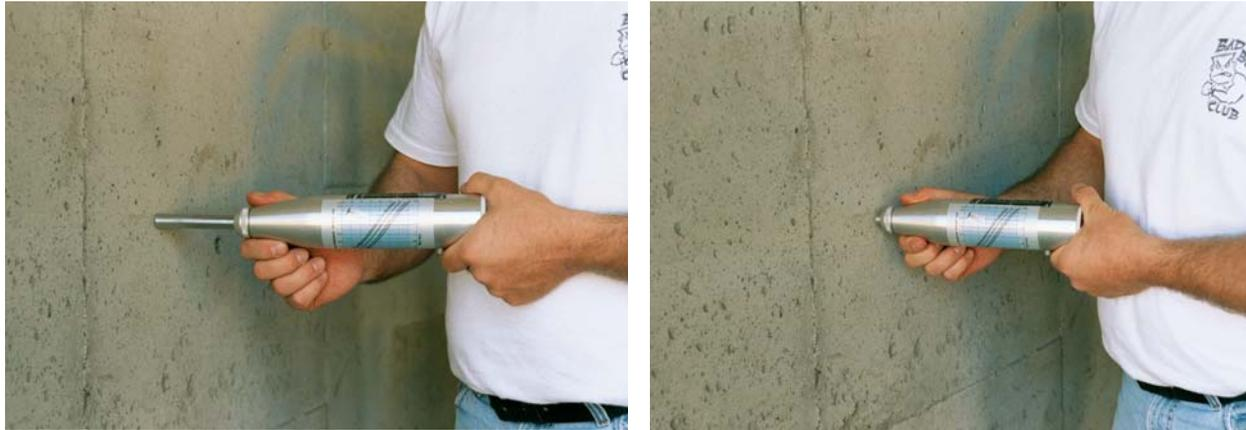
Figures 1 and 2 – Horizontal orientation of hammer during a measurement
