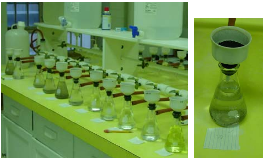
Figure 6.7 – Filtering of samples to remove HCl, CaCl 2 and leached carbonates.
