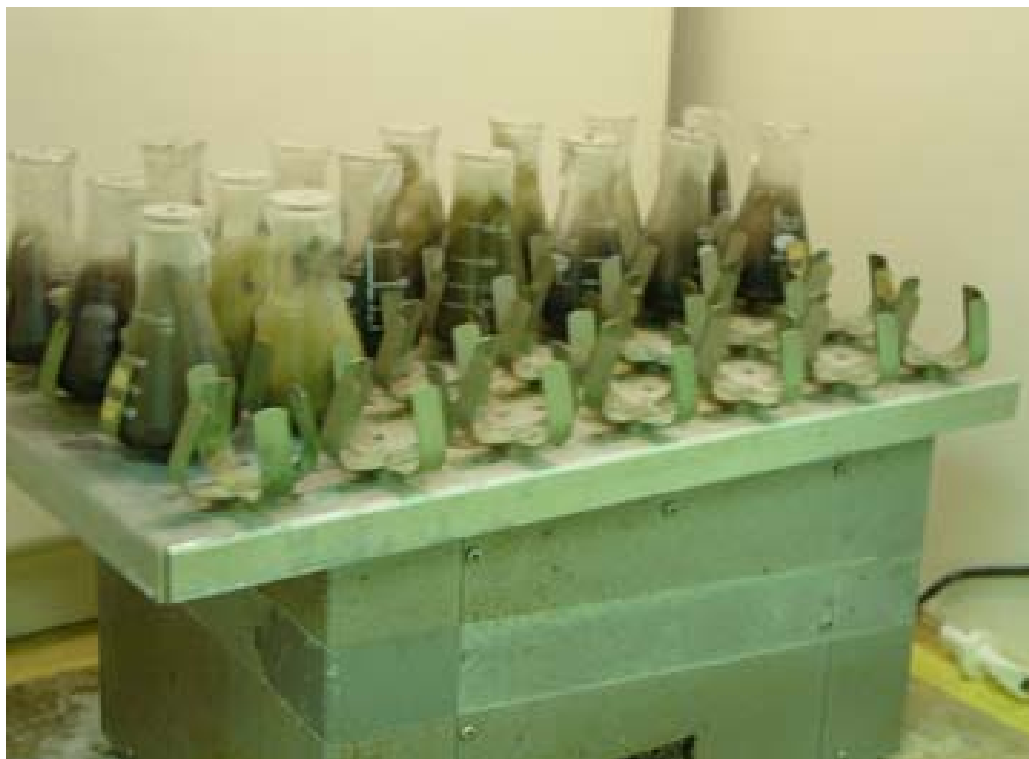
Figure 6.6 - Agitation of samples leached with HCl to remove carbonates.
