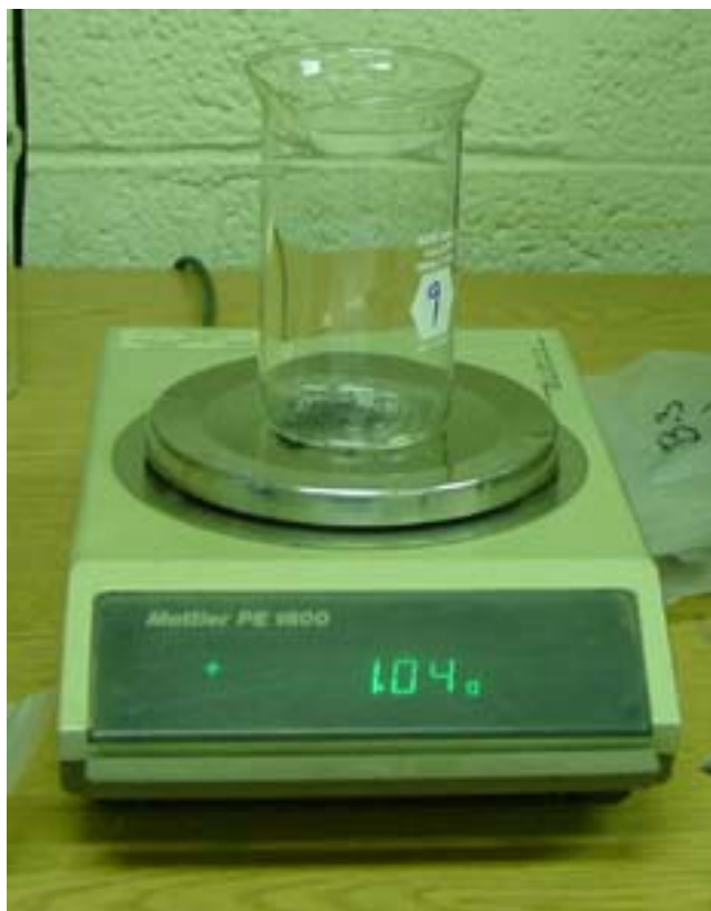
Figure 6.8 - Weighing of 1g sample for \text{H}_2\text{O}_2 oxidation testing.
