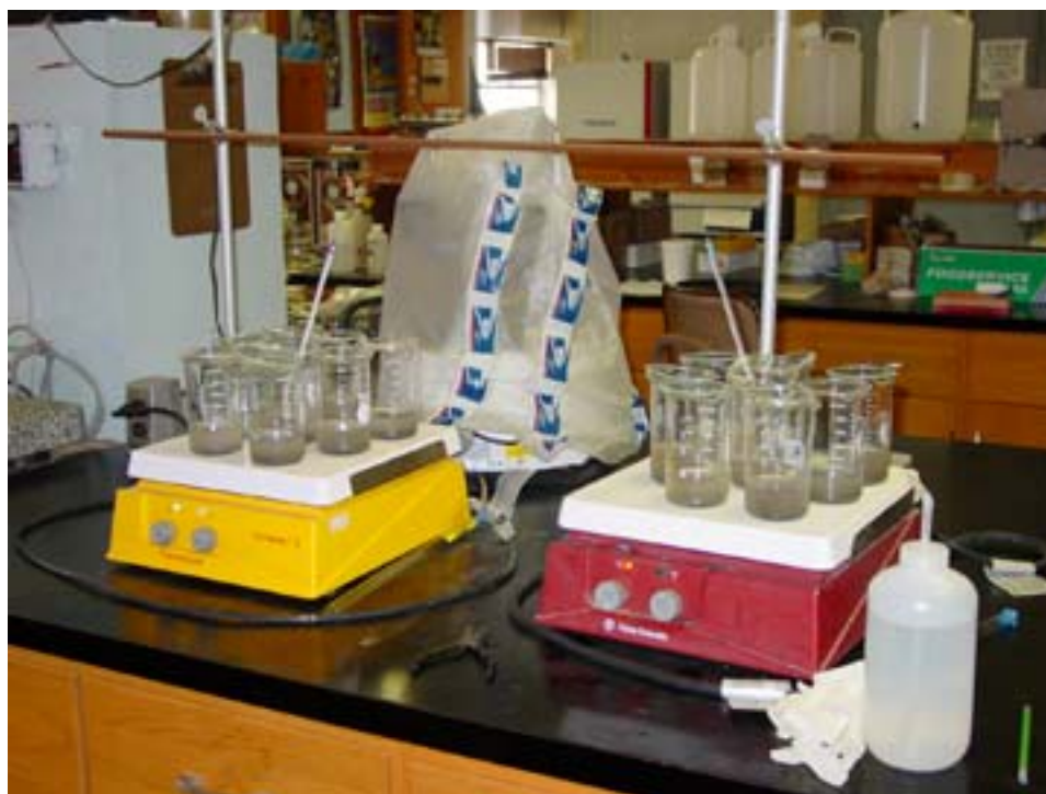
Figure 6.10 - Samples on hotplate ( 95^\circ\text{C} ) to boil off excess \text{H}_2\text{O}_2 .
