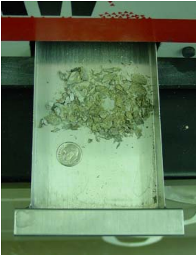
Figures 6.2 and 6.3 – (6.2) Spex 4200 Jaw Crusher. (6.3) Size of rock fragments obtained by passing sample through Jaw Crusher.
