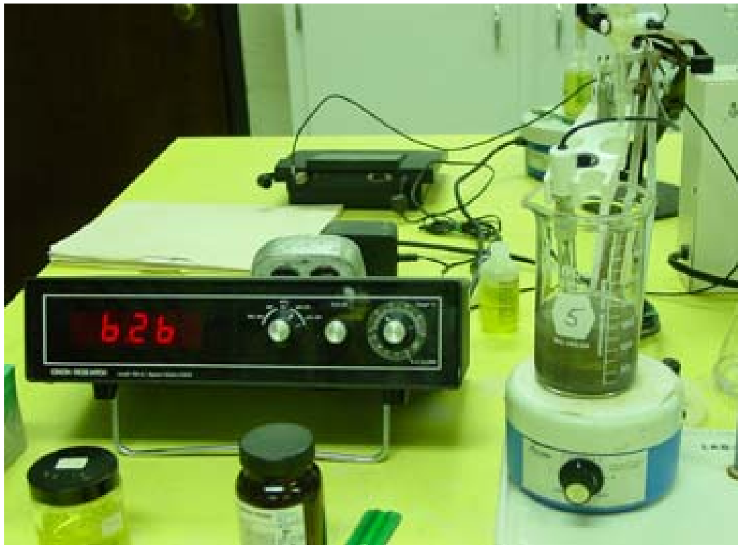
Figure 6.23 - Determination of pH using combination electrode and digital pH meter.
