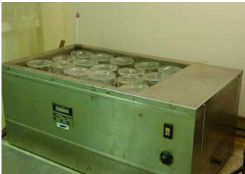
Figure 6.9 - Sixteen samples in hot water bath ( 50^\circ\text{C} ) while being oxidized with hydrogen peroxide ( \text{H}_2\text{O}_2 ).
