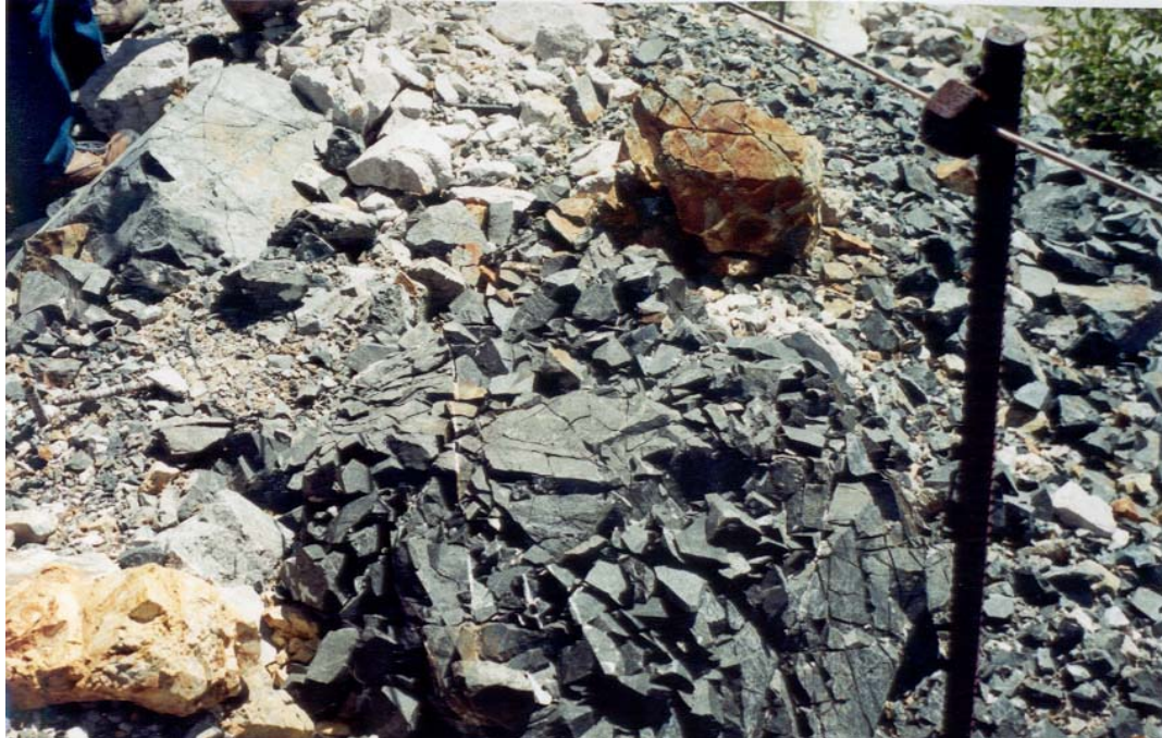
Figure 5.8 – Significant aggregate weathering at the Questa mine waste piles site. Photo from Dr. James K. Mitchell.
