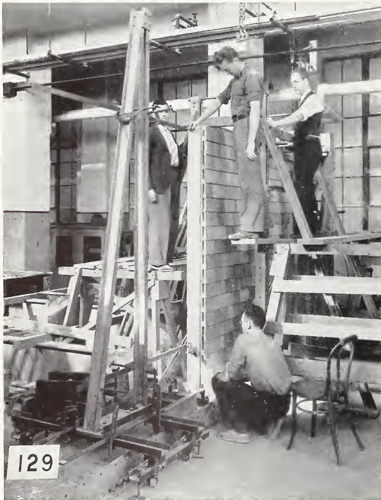
FIGURE 69.—Wall specimen BL-R1 under racking load.
