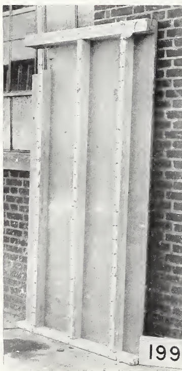
FIGURE 1.—Frame of wall specimen BK-14.
