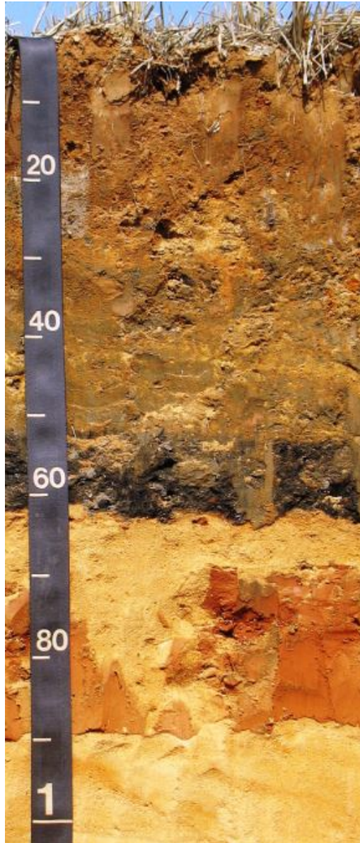
Profile of a Virginia soil that formed in human-transported material. The upper 52 cm was deposited by truck from nearby sources of fill material and contains scattered broken peds of diagnostic horizons that formed at their original locations. The dark layer at a depth of 60 cm has a high content of wood and coal ash. The lower part of the profile consists of deposits of dredged marine sediments. Scale is in cm. (Photo courtesy of Dr. John Galbraith)
