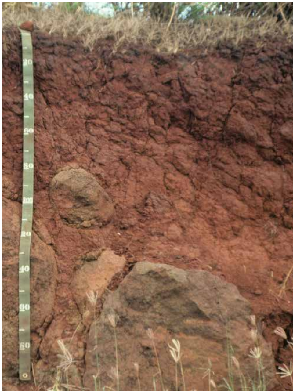
Profile of a Torrox (specifically a Haplotorrox) in Hawaii. This soil formed in residuum from a basaltic lava flow. Scale is in cm.
