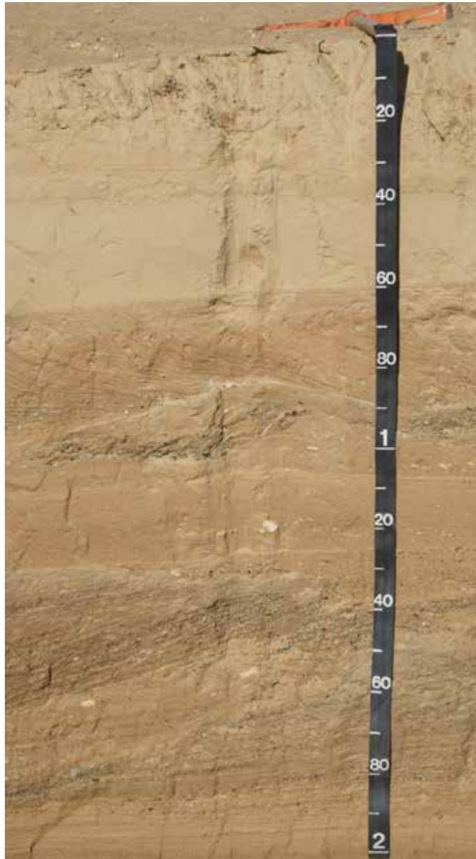
Soil profile (of a Torriorthent in the United Arab Emirates) showing rock structure as fine to coarse stratifications throughout. The upper 60 cm is recent eolian sand. The lower part consists of old alluvial deposits interspersed with eolian strata. Scale is in cm. (Photo courtesy of Dr. Craig Ditzler)
