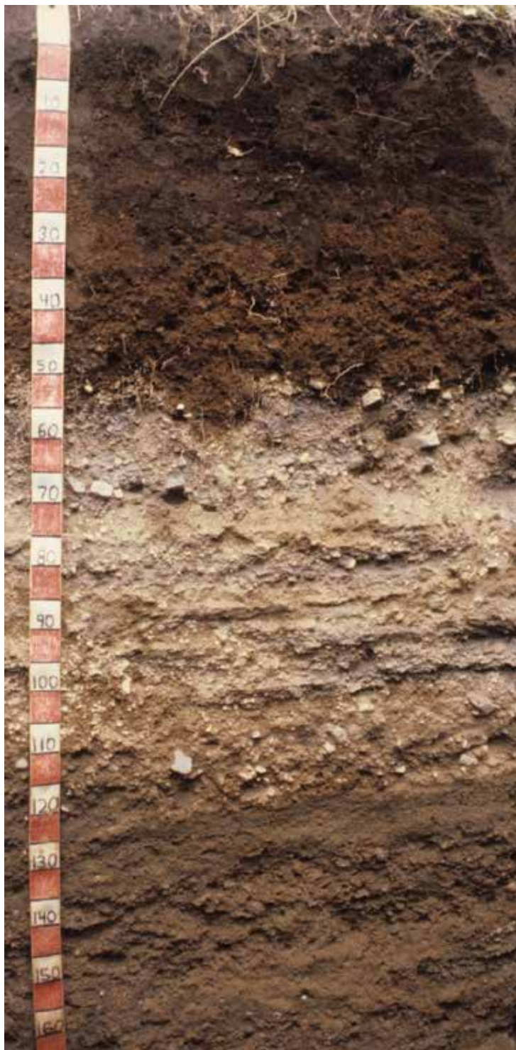
Profile of a Vitrand (specifically an Ustivitrando) in the Philippines. This soil has an umbric epipedon. Scale is in cm.
