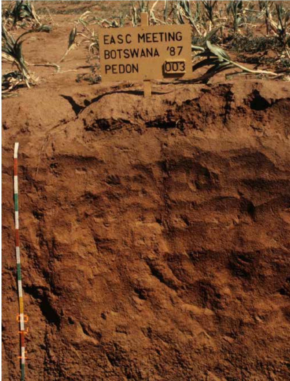
Profile of an Ustalf (specifically a Paleustalf) in Botswana. The soil has a thick clayey argillic horizon beginning at a depth of about 10 cm and extending beyond the base of the photo. Scale is in 10-cm increments.
