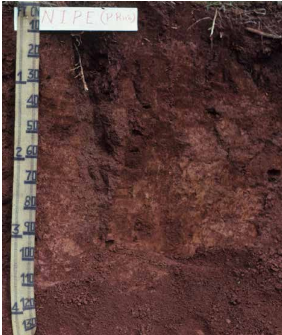
Profile of a Udox in Puerto Rico. This soil is an Acrudox and therefore has a very low nutrient-holding capacity.
