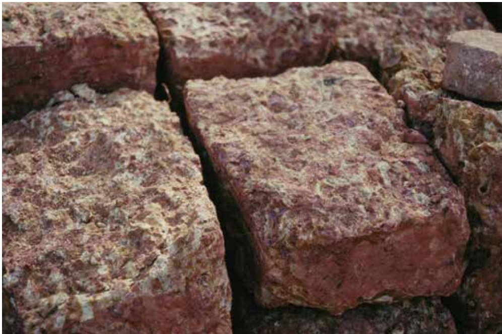
Bricks made by hand from dried, plinthite-rich soil material (India).
