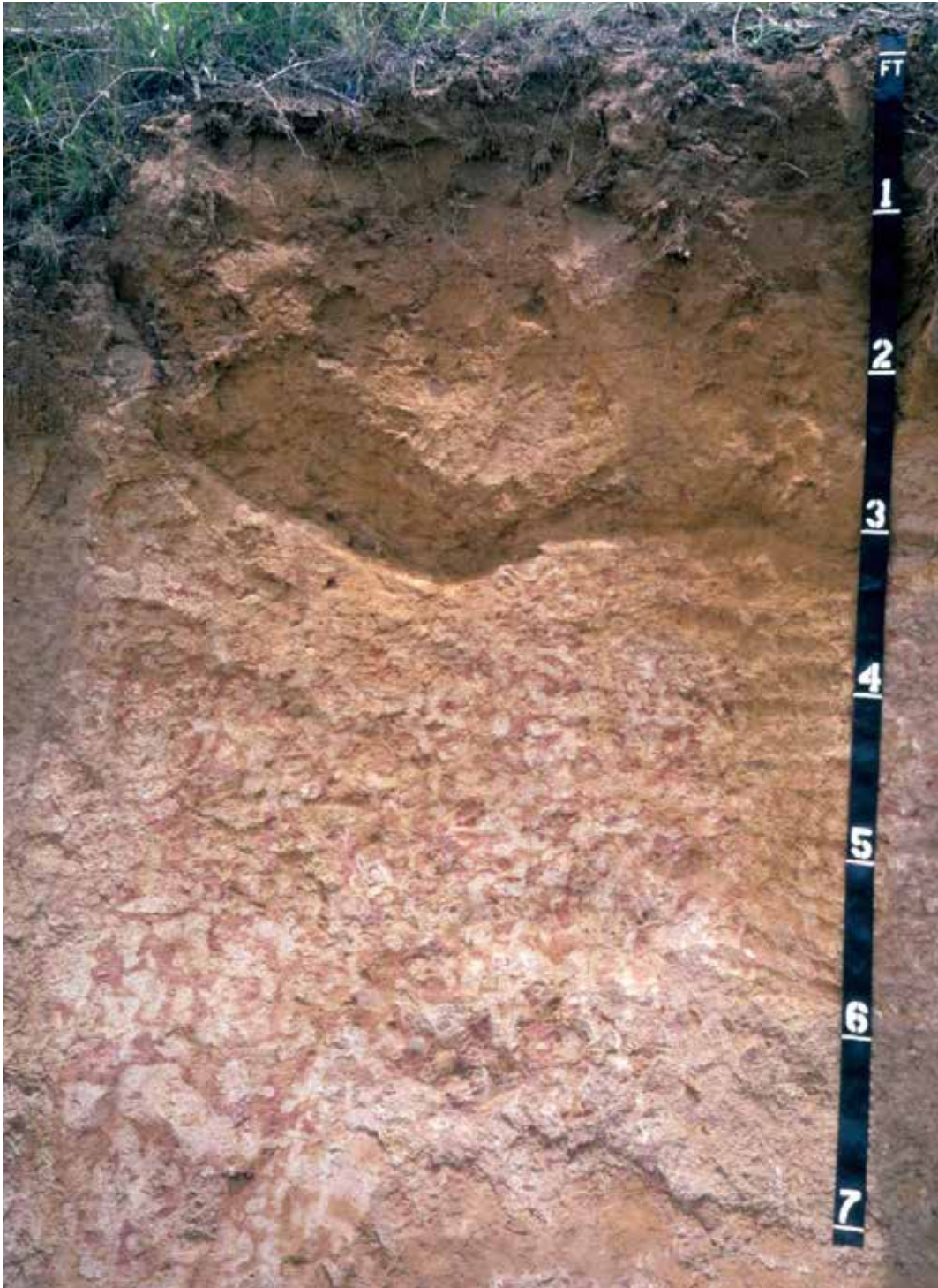
Profile of a Kanhapludult in Georgia. It has an ochric epipedon about 12 inches thick underlain by a reddish yellow kandic horizon that extends to a depth of about 36 inches. Below the kandic horizon is weathered granitic saprolite. Scale is in feet.
