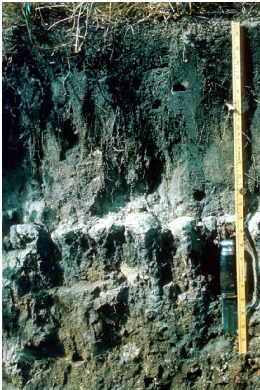
Profile of a Cryoll (specifically a Natricryoll). The soil has a natric horizon below a depth of 14 inches. Scale is in inches.
