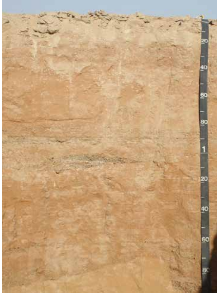
Profile of an Aridisol (specifically a Haplocalcid) in the United Arab Emirates. White concentrations are calcium carbonate masses. Scale is in cm. (Photo courtesy of Dr. Craig Ditzler)
