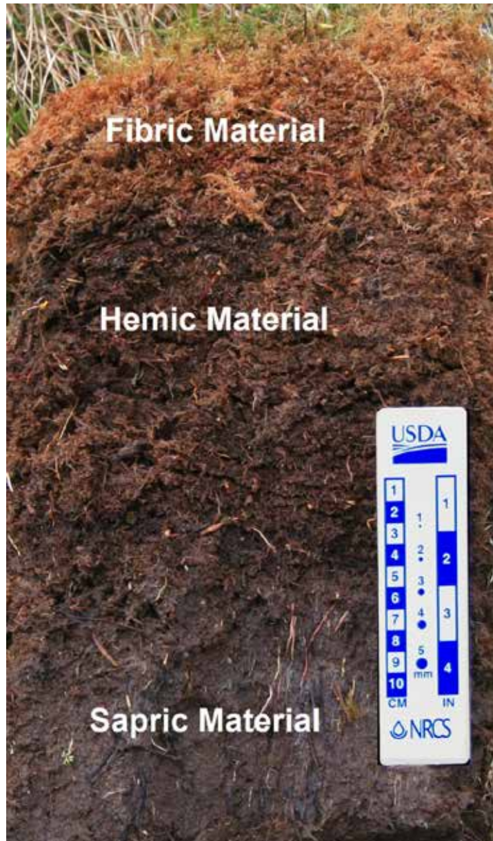
Organic soil materials, including fibric (top), hemic (middle), and sapric (lower) materials. (Photo courtesy of John Kelley)
