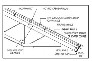
B. Starting at low or outside edge of the roof, place the panel on the bar joists with groove edge toward low portion of roof and tongue toward high portion. Fasten using Olympic #14-10 Heavy All Purpose screws (or equal) 1-1/2" from edges and one in the center (12" from edge at each bar joist location (3 screws per joist), see diagram on top of page 2. To install pre-drill hole through panel into flange of the steel joist using 7/32" high-speed
