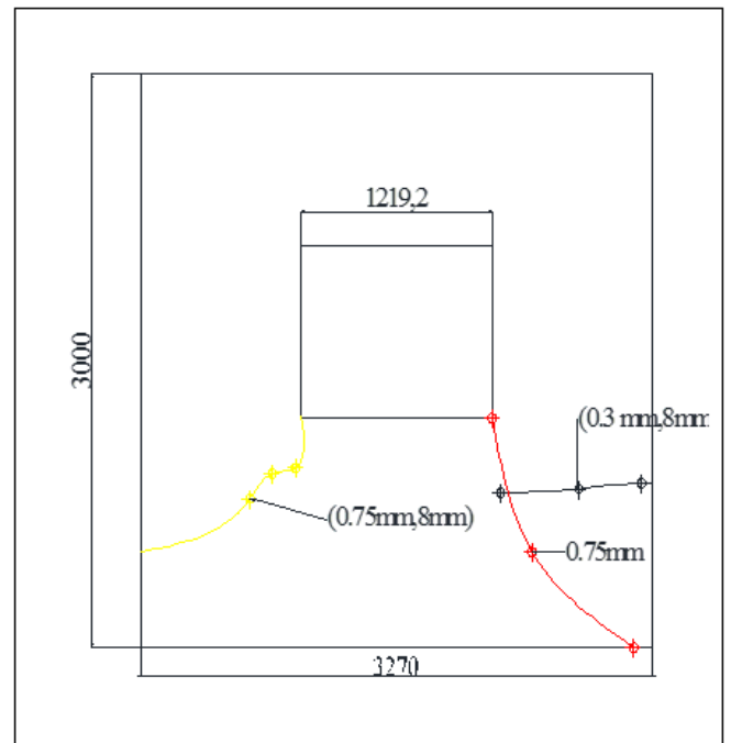
Figure: 8 Crack profile for Master bedroom wall 1
