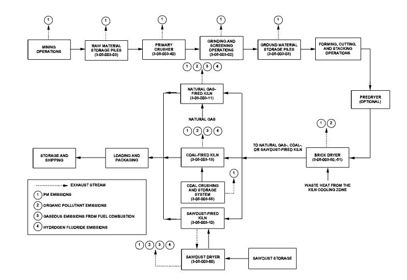
Figure 11.3-1. Typical brick manufacturing process. (Source Classification Codes in parentheses.)
