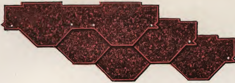
The 10 1/2" Hexagonal Shingle provides a minimum headlap of 2 1/2". Note the dove-tailing joints at the ends of the strips.
