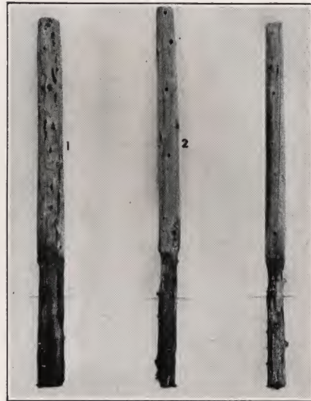
Untreated cedar fence posts, after being in service nine years. In each case the sapwood was entirely gone; in post No. 1 about one-third of the entire bottom rotted away; in post No. 2 one-half of the bottom decayed, while in post No. 3 more than one-half of the bottom decayed. Carbosota would have prevented this condition. (Photo courtesy Iowa State College of Agriculture.)
