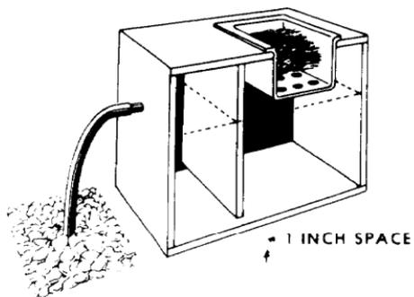
Grease trap--Used with both soakage pit and trench to prevent clogging of the soil.
