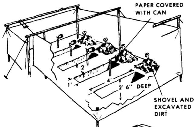
Deep pit latrine--Used for longer periods of time and in build up areas. Collapsible 2-seat boxes are available in the supply system.
