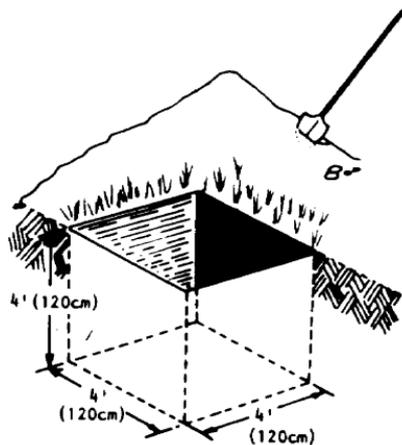
Soakage pit/trench--Used to prevent accumulation of liquid waste (water from showers, sinks, and field kitchens).
