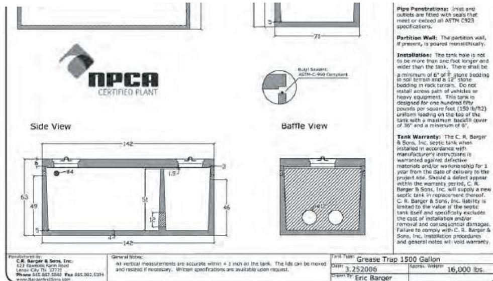
A typical 1,500 gallon (5,680 L) non-traffic-rated tank with monolithic partition wall was chosen as the test subject for analyzing how non-traffic-rated tanks perform under live vehicle loading (Figure 1). This example is an actual precast concrete tank design that has been in use for more than 15 years as a non-traffic-rated tank. The lid thickness is 6 inches (150 mm) with an average wall thickness of 4 inches (100 mm) and a bottom slab thickness of 4 inches.
