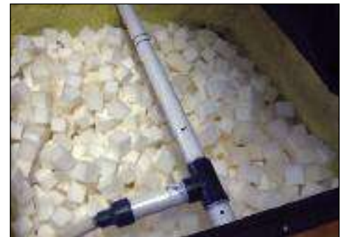
Synthetic media — foam cubes (top view).
