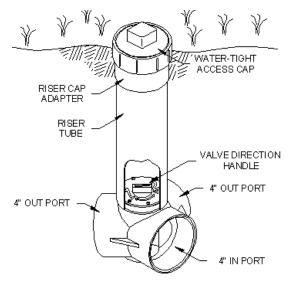
The Bull Run Valve is available in 4" sch 40 pvc and is suitable wherever septic disposal systems are used - in commercial, industrial, and residential applications.
