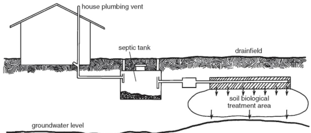
septic system. If the water table is at least 3 feet below the top of the septic tank but the drainfield still is flooded or saturated, then you may use your septic tank as a holding tank. Have it commercially pumped, but don't pump out more than half of the volume of the tank.
