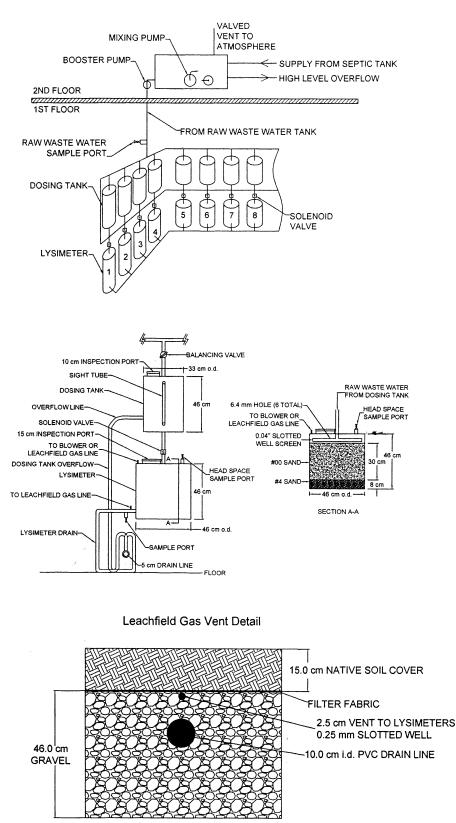
Fig. 1. Schematic diagram of experimental facility (top), lysimeters (middle), and detail of leachfield gas intake (bottom). Drawings are not to scale.
