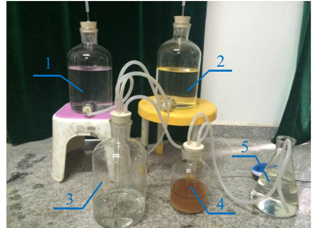
Fig. 4. Simulated BSA corrosion device without specimens, 1-Na 2 S solution, 2-HCl solution, 3-H 2 S reaction bulb, 4-Medium erosion liquid, 5-Water.
