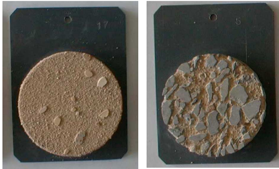
Fig. 8. A sample of the centrifuged concrete P2-I-G (left) and of concrete P3-I52.5-G (right) produced by hardening in the form after four cycles of the microbiological test.
