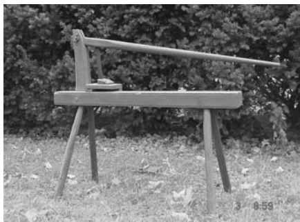
Fig. 5. An antique hole punch from the collection of John Fugelso. A hole punch is used to make the nail hole in each shingle.
