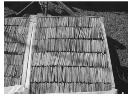
Fig. 10. A delivery crate packed tightly with banded bundles, arranged by size, of new red oak shingles for use at the Wright's Ferry Mansion, in Columbia, Pennsylvania.
