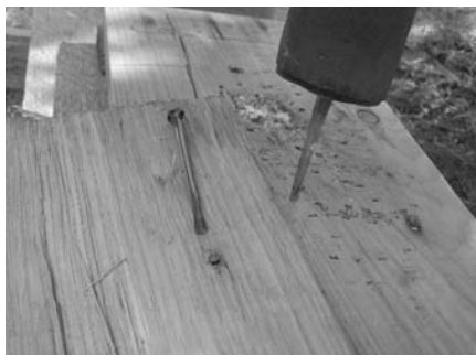
Fig. 6. A spade-pointed nail and freshly punched shingle; the working end of a hole punch is at the right.
