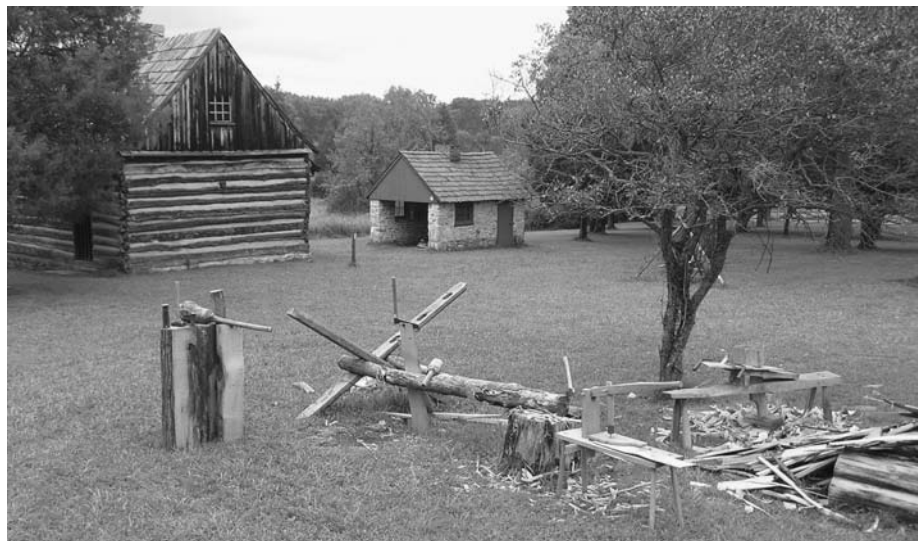
Fig. 3. An array of tools used to make shingles, left to right: wedges and a small sledge; a maul and gluts, on a halved shingle log; riving brake with a shingle bolt, mallet, and froe; hole punch with a shingle under the retainer, ready to punch; a shaving bench and drawknife with a shingle clamped under dumb head; and the scrap pile. Bertolet House, the larger log building in the background, was reroofed in 2007.
