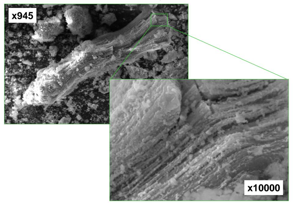
TEM of a thermally treated chrysotile bundle showing a complete recrystallization of the original fibres into newly-formed high temperature silicates
