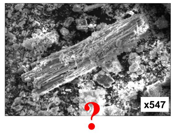
•At low magnification the microstructure of a thermally treated fibre is not revealed and doubts may arise on the effectiveness of the thermal treatment. At higher magnification the issue may be unravelled
