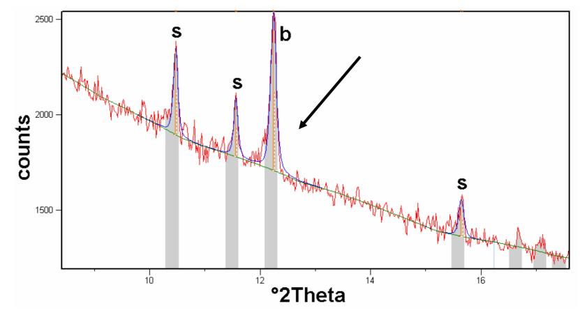
Low angle region of powder pattern of a sample of cement-asbestos slate fired at 1200 °C with the presence of the brownmillerite (**b**) and silicocarnotite (**s**) peaks
