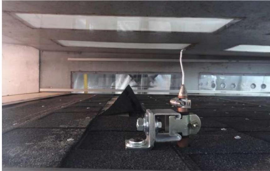
Figure 6-7. Interior view of the DFS during this study's wind test. A partially unsealed laminate shingle instrumented with load cells is shown.
