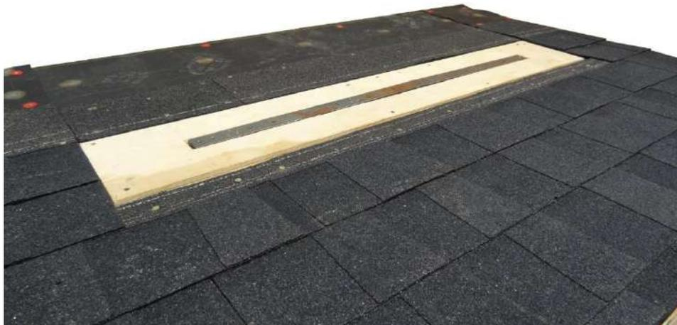
Figure 6-15. Part 2: load cell arrangement for Laminate specimen showing wood decking surrounding top plates.
