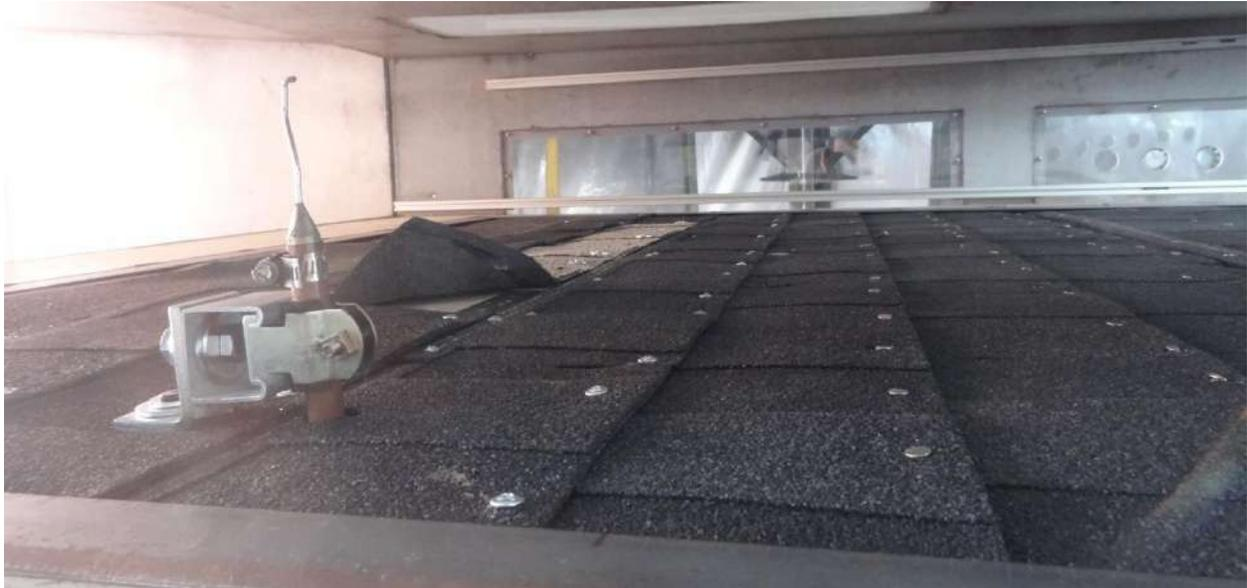
Figure 6-33. Partially unsealed Laminate Specimen 3 lifting in 44 m/s (98 mph) mean wind velocity.
