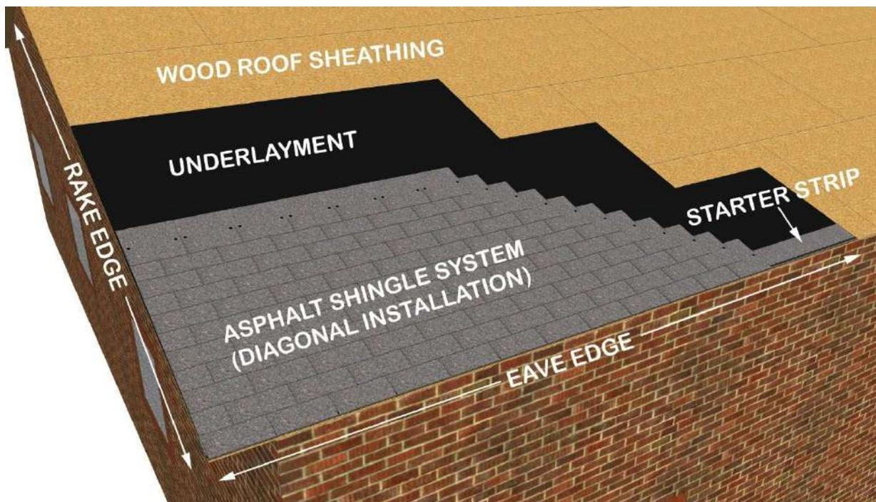
Figure 2-7. Diagonal installation of three-tab asphalt shingle system. Laminate installation produces a similar pattern.
