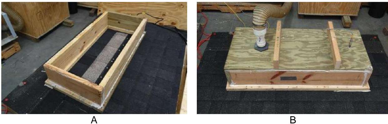
Figure 6-28. Phase II experimental setup. A) Laminate specimen with pressure box. B) Sealed box with air hose and pressure sensor attached.
