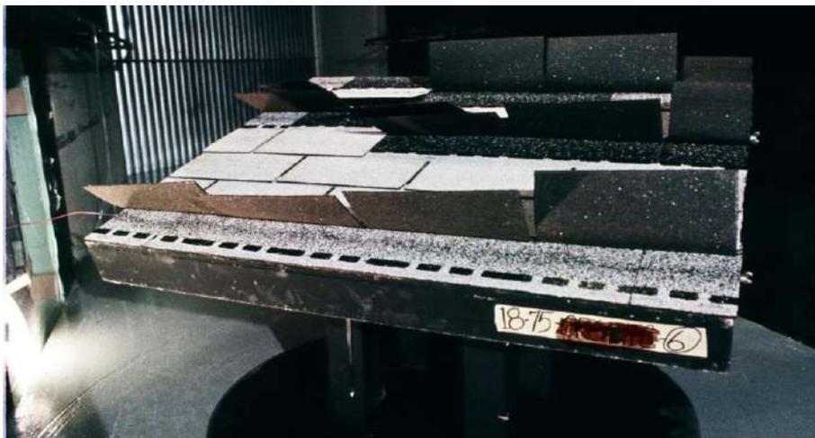
Figure 3-2. Post-wind test asphalt shingle test deck inside the Colorado State University Meteorological Boundary-Layer Wind Tunnel (Figure courtesy of Jon Peterka)
