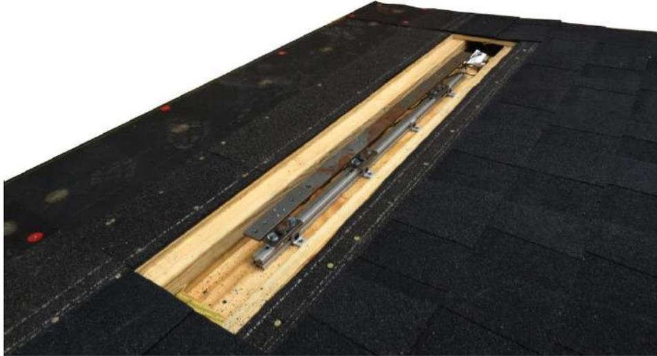
Figure 6-14. Part 1: load cell arrangement for Laminate specimen showing load cell base connection.
