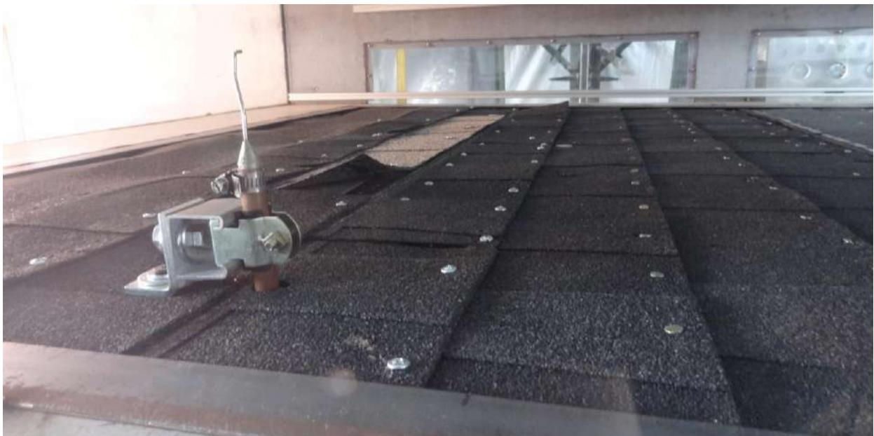
Figure 6-34. Partially unsealed Laminate Specimen 4 lifting in 44 m/s (98 mph) mean wind velocity.
