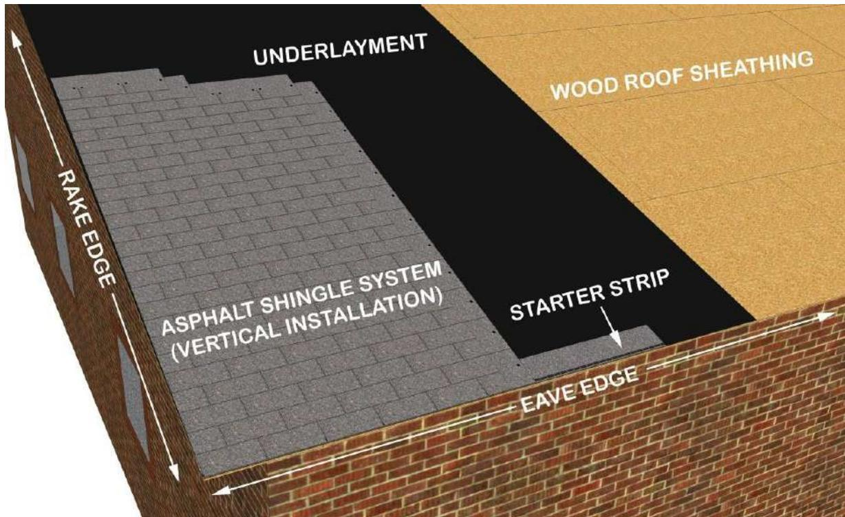
Figure 2-8. Vertical (racked) installation of three-tab asphalt shingle system. Laminate shingles are not installed with this pattern.
