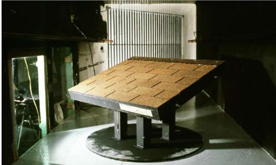
Figure 3-1. Pre-wind test asphalt shingle test deck inside the Colorado State University Meteorological Boundary-Layer Wind Tunnel (Figure courtesy of Jon Peterka)
