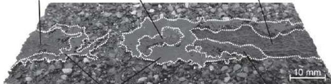
Sealant Strip-to-Top Shingle Adhesive Failure
