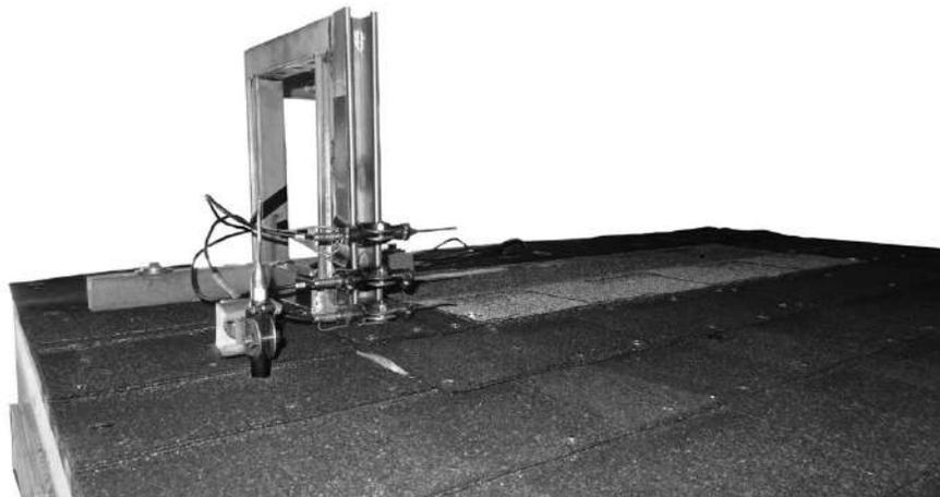
Figure 6-22. Velocity sensor test setup.
