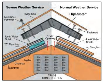
Can be used with Blue and Red label No.1 and No.2 Fivex-Perfections-Royal shingles. Adapts to ridge pole or truss construction.
