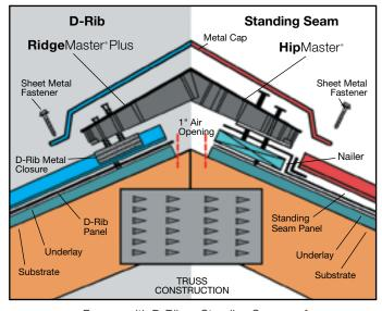
For use with D-Rib or Standing Seam roofs. Adapts to ridge pole or truss.
