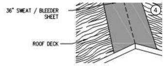
b. Install Ribbed Valley Metal on top of the sweat/bleeder sheet in the center of each roof valley. (Figure 5)
