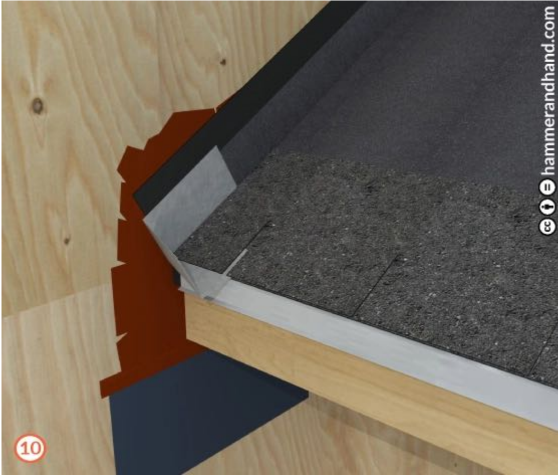
Install first course of shingles.
