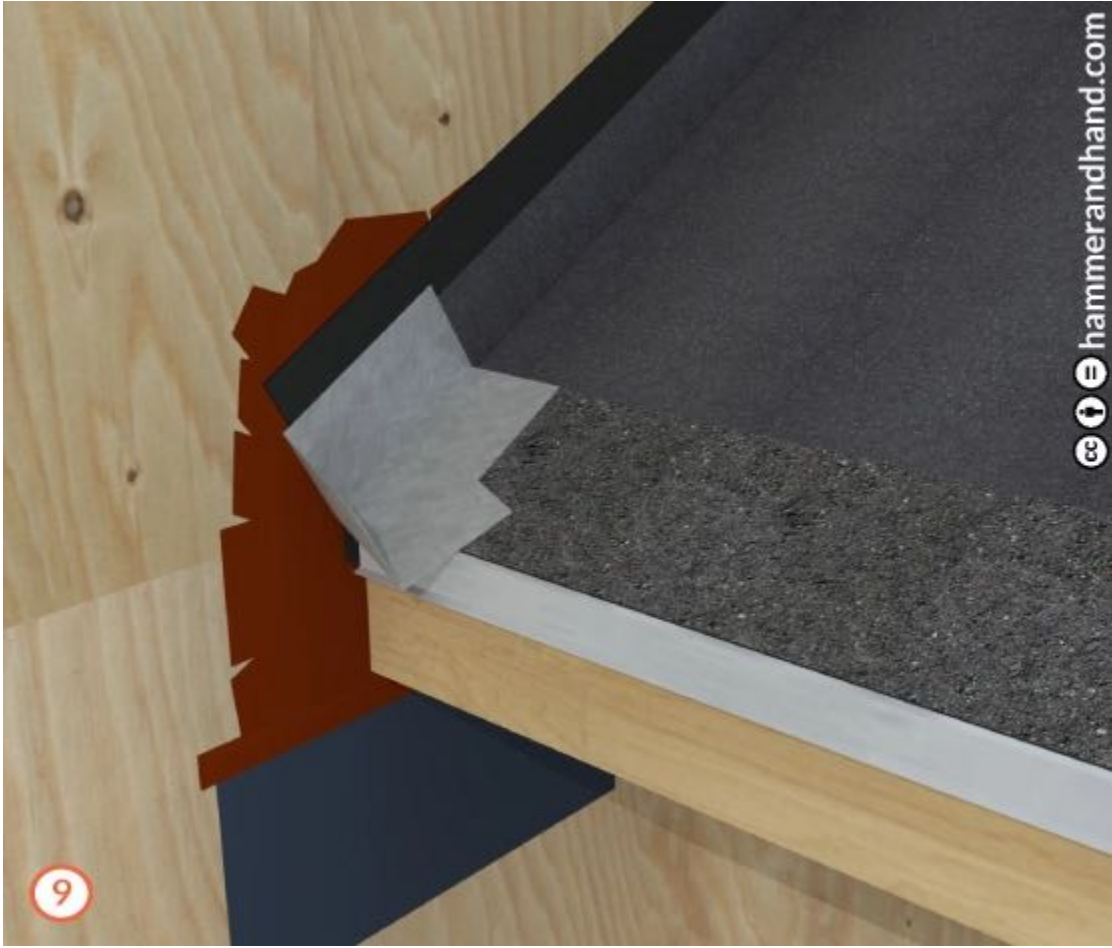
Fasten kick flashing in upper right corner.
