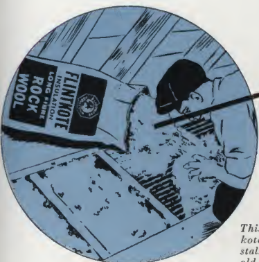
Flintkote Rock Wool Bats fill hollow walls and attic spaces to a uniform thickness and density.
