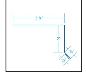
EF-3 Eave Flashing is used with: Gibraltar 2 1/2" Corrugated Panels
