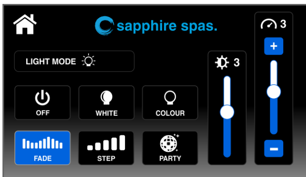
Fade Effect Fade transition through all possible colours Light effect transition speed (RH slider) Light brightness adjustment (LH slider)
