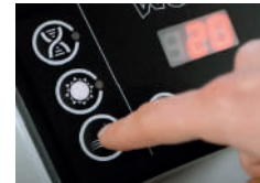
4. Connect the pump unit then press the button to inflate the spa. The air flow valve prevents your spa from over-inflating
