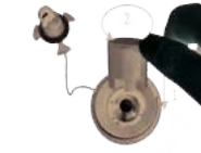
Use tools to unscrew air valve spindle.
