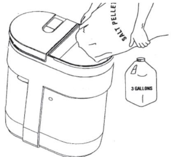
ADDING SALT TO THE BRINE CABINET
