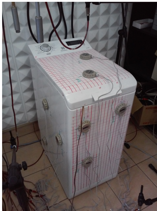
Figure 1: A photograph of the washing machine casing with attached actuators.
