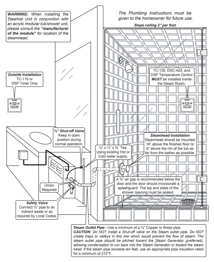
Figure 3: Typical installation
