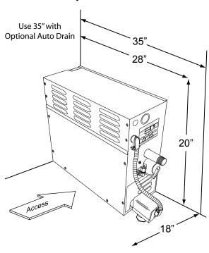
Select a location for mounting the Steam Generator that is accessible for installation and service. The access requirement indicates the minimum space for convenient access to Steam Generator.
